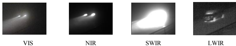
Fig. 10. Images showing the glare effect in the VIS, NIR and SWIR spectral bands
