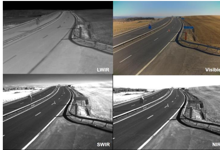
Fig. 3. Example of snapshots recorded by LWIR (top left), Visible (top right), SWIR (bottom left) and NIR (bottom right) cameras
