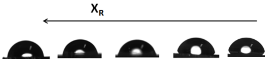
Figure 1: Hydrophilicity of ICO nanofilms by water contact angle measurements for films with different X_R ratios. From right ( X_R=0.33 ) to left ( X_R=1 ) the silica to castor oil ratio is increased.
