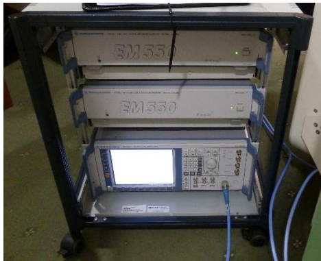
Fig. 2.1.2. Testbed for measurements of off-body channels with antenna diversity
