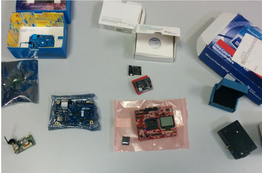
Fig. 3.5.1. On the bottom left, a wireless sensor node. Intel Galileo board is at the center-left. TI MSP430 experimental kit is at the center-right. Right over that, TI sensortag is placed. Raspberry Pi is in a black case at the bottom right.
