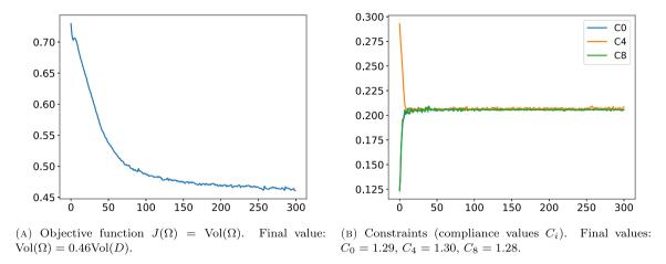
FIGURE 13. Convergence history curves for the three load case of Section 6.2.1.
