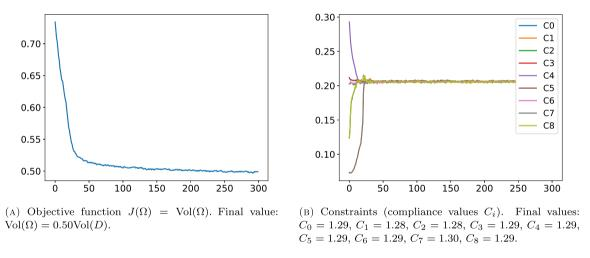
FIGURE 14. Convergence history curves for the nine load case of Section 6.2.1.
