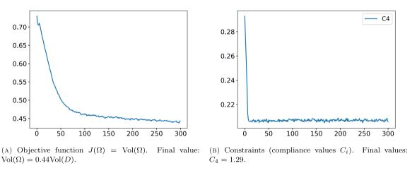
FIGURE 12. Convergence histories for the single load case of Section 6.2.1.
