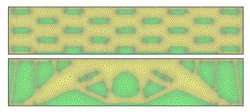
FIGURE 10. Meshes of the initial and final shapes for the nine load case of Figure 9c (Sect. 6.2.1).
