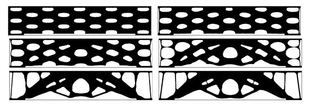
FIGURE 11. Intermediate minimizing shapes for the nine load case of the volume minimization problem of Section 6.2.1 (iterations 0, 5, 10, 20, 80, and 300).
