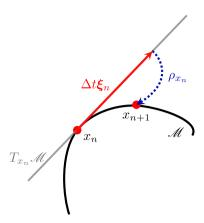
FIGURE 2. Optimization on a manifold  $\mathcal{M}$ : a retraction map  $\rho_{x_n}$  is used to project a tangential motion  $\Delta t \boldsymbol{\xi}_n \in T_{x_n} \mathcal{M}$  from  $x_n \in \mathcal{M}$  back onto the optimization domain  $\mathcal{M}$ .
