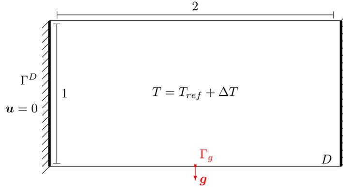
FIGURE 3. Setting for the thermoelastic compliance minimization problem of Section 6.1, issued from [64].
