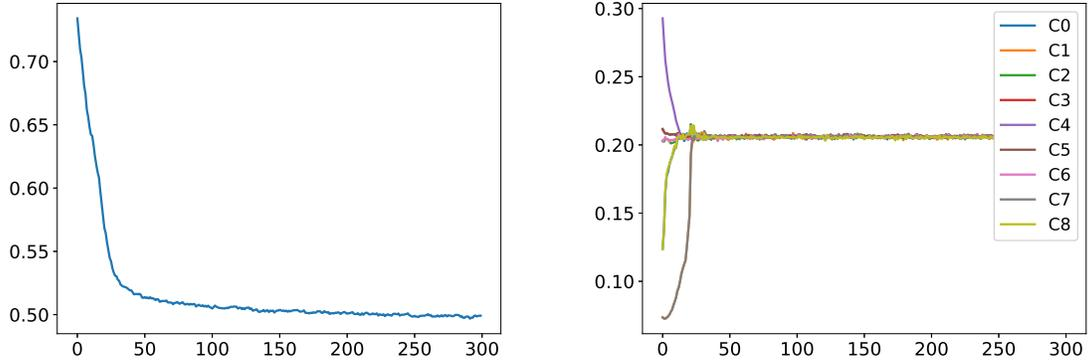
(A) Objective function  $J(\Omega) = \text{Vol}(\Omega)$ . Final value:  $\text{Vol}(\Omega) = 0.50\text{Vol}(D)$ . (B) Constraints (compliance values  $C_i$ ). Final values:  $C_0 = 1.29, C_1 = 1.28, C_2 = 1.28, C_3 = 1.29, C_4 = 1.29, C_5 = 1.29, C_6 = 1.29, C_7 = 1.30, C_8 = 1.29$ .
