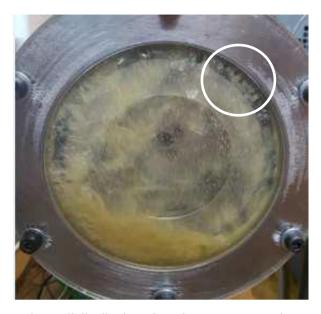
Fig. 5 Oil distribution when planets are mounted on carrier. The oil pocketing is highlighted in the white circle
