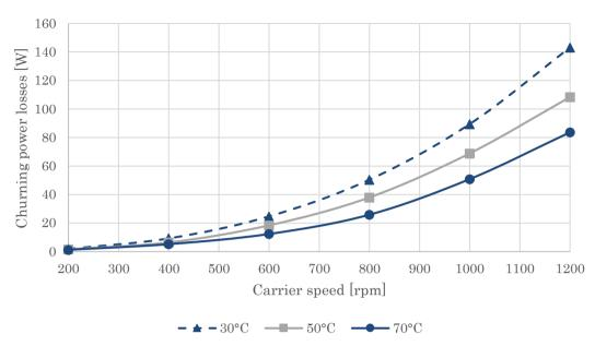
Fig. 7 Churning losses of the planet-carrier regarding the carrier speed and oil sump temperature for a dynamic oil level of 24mm
