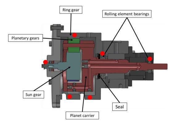
Fig. 2 Transmission section (temperature probes locations are plotted as red dots)
