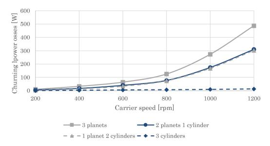
Fig. 10 Churning losses for different planets number regarding the carrier speed for a dynamic oil level of 6.5mm and an oil sump temperature of 30°C
