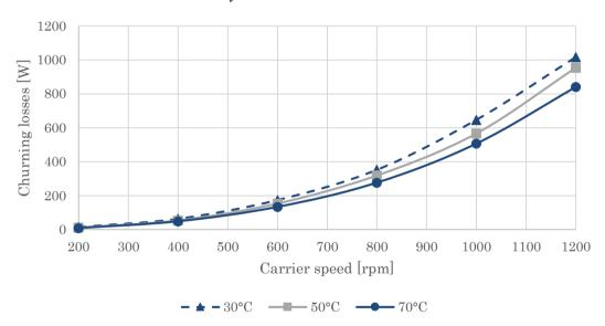
Fig. 8 Churning losses when three planets are mounted on the carrier regarding the carrier speed and oil sump temperature for a dynamic oil level of 24mm
