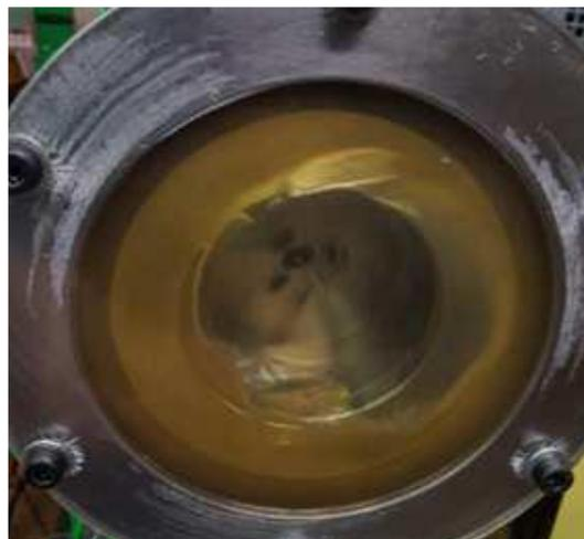
Fig. 4 Oil flow around the planet-carrier. The oil ring can be observed on the periphery due to centrifugal effects
