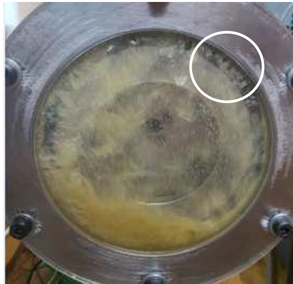
Fig. 5 Oil distribution when planets are mounted on carrier. The oil pocketing is highlighted in the white circle
