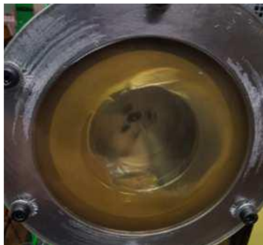
Fig. 4 Oil flow around the planet-carrier. The oil ring can be observed on the periphery due to centrifugal effects
