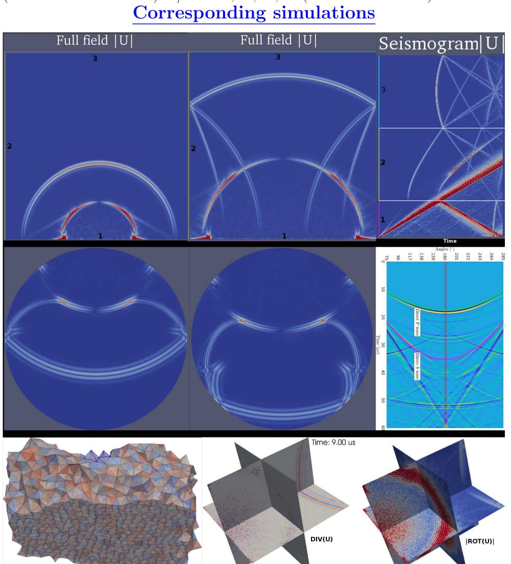
Corresponding 2D and 3D simulations by Finite Element method featured with IPDG[1]. The 3D simulation is performed in a reduced model with Absorbing Boundary Conditions due to memory limits.
