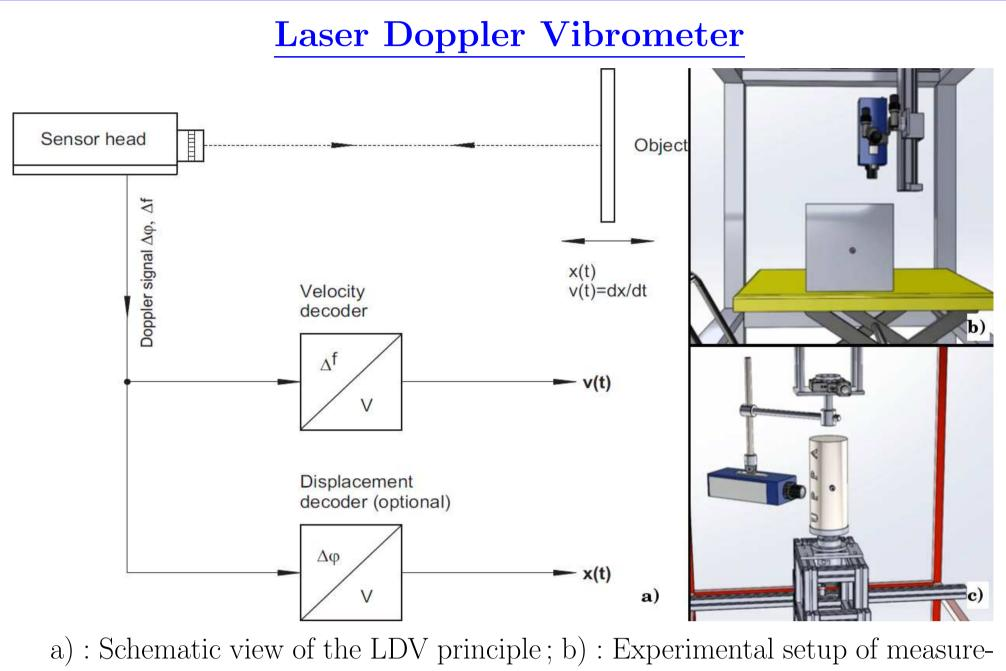
ments on an Alu block by a single point LDV sensor. c): Experimental setup for the Alu cylinder.
