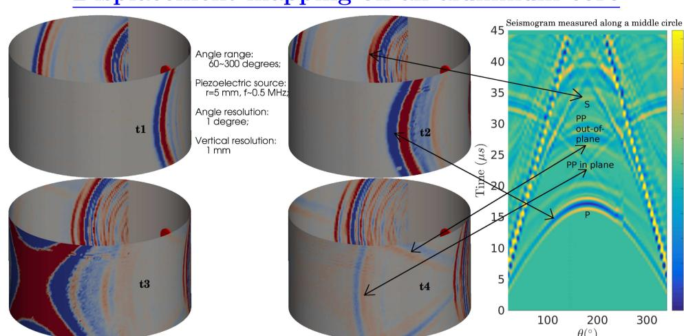
Radial components of displacements are measured. Snapshots and seismogram (around the mid-section) at/until t1, t2, t3, t4 (t1 < t2 < t3 < t4) are shown.
