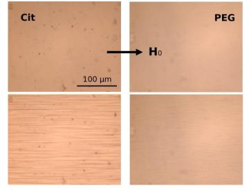
**Figure 1**. Snapshots of aqueous suspensions of citrated (left) and PEGylated (right) MNPs at  $\varphi_0$ =0.13% submitted to  $H_0$ =13.5 kA·m<sup>-1</sup> at t=0 (upper row) and 5 min after field application (bottom row).
