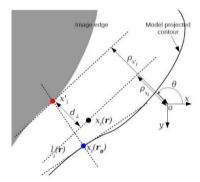
Fig. 3. Contour tracking for the pose estimation, extracted from [26]. From the initial pose  $r_0$ , a one-dimensional search is performed along the normal to the projected contour underlying the measurement point  $x_i$  ( $r_0$ ). And minimizing the distance d between the point  $x'_i$  and the line  $l_i(r)$ .
