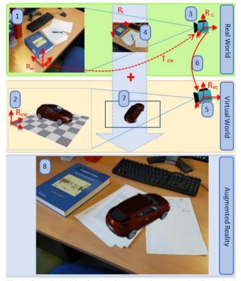
Fig. 1. General principle of registration process in augmented reality. 1) Real environment. 2) Virtual environment. 3) Camera. 4) Captured image. 5) Virtual camera. 6) Alignment of the virtual camera with the actual camera. 7) Projection space. 8) Augmented reality.
