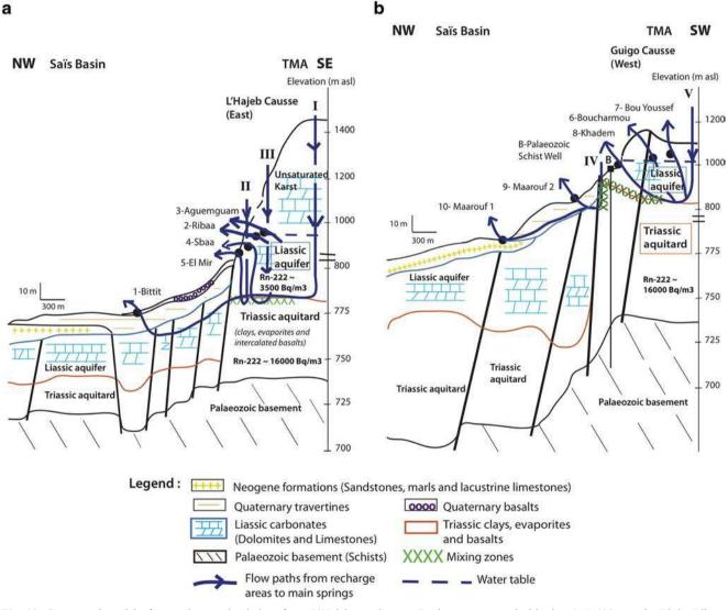
Fig. 10 Conceptual model of groundwater circulation, for a L'Hajeb Causse in the east, and for b Guigo Causse in the west, with mixing zones between the Middle Atlas Causses and Saïs Basin, from five recharge areas to springs—I to III: L'Hajeb Causse; IV, V: Guigo
