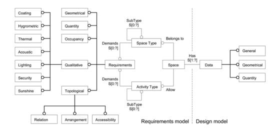
Figure 3 Schema of space data model. including identified qualitative and topological requirements
