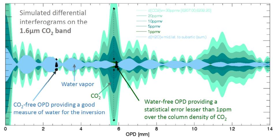
Figure 3. Jacobian interferograms (arbitrary unit) when varying the CO<sub>2</sub> or H<sub>2</sub>O concentration<sup>13</sup>. During the design phase of Nanocarb, the choice of the measured OPD will be done taking into account the impact of other species than CO<sub>2</sub>.
