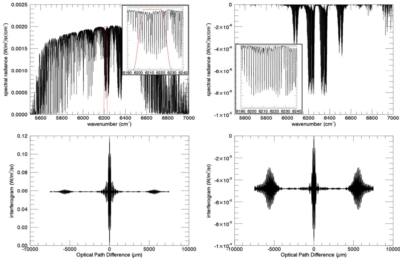
Figure 2. Typical radiance simulated with Modtran for a spaceborne mission viewing at nadir. Top: spectra; bottom: corresponding interferograms after filtering between 6200 cm<sup>-1</sup> and 6225 cm<sup>-1</sup> (red curve). Left: total radiance with a CO<sub>2</sub> concentration of 400 ppm; right: difference between the radiance with 405 ppm and with 400 ppm of CO<sub>2</sub>, the other parameters being unchanged.
