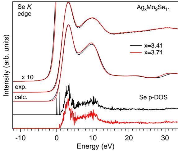
FIG. 10: Experimental Se  $K$  XAS spectra of  $\text{Ag}_x\text{Mo}_9\text{Se}_{11}$  for  $x=3.41$  and  $x=3.71$  compared to calculated spectra and unoccupied Se  $p$ -DOS of  $\text{Ag}_x\text{Mo}_9\text{Se}_{11}$  for  $x=3.5$  and  $x=4.0$ , respectively.
