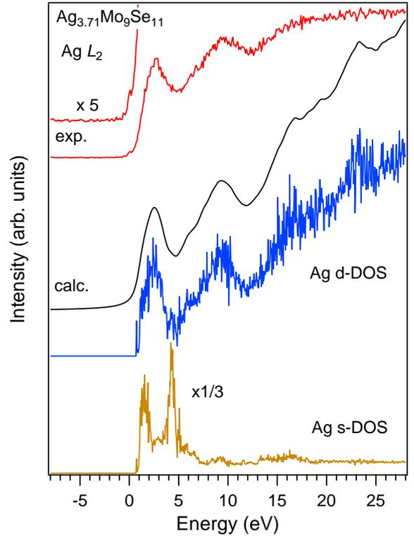
FIG. 9: Experimental Ag  $L_2$  XAS spectrum of  $\text{Ag}_{3.71}\text{Mo}_9\text{Se}_{11}$  compared to the calculated spectrum and unoccupied Ag  $d$ - and  $s$ -DOS of  $\text{Ag}_{4.0}\text{Mo}_9\text{Se}_{11}$ . The calculated spectrum is obtained by broadening the Ag  $d$ -DOS to account for experimental resolution.
