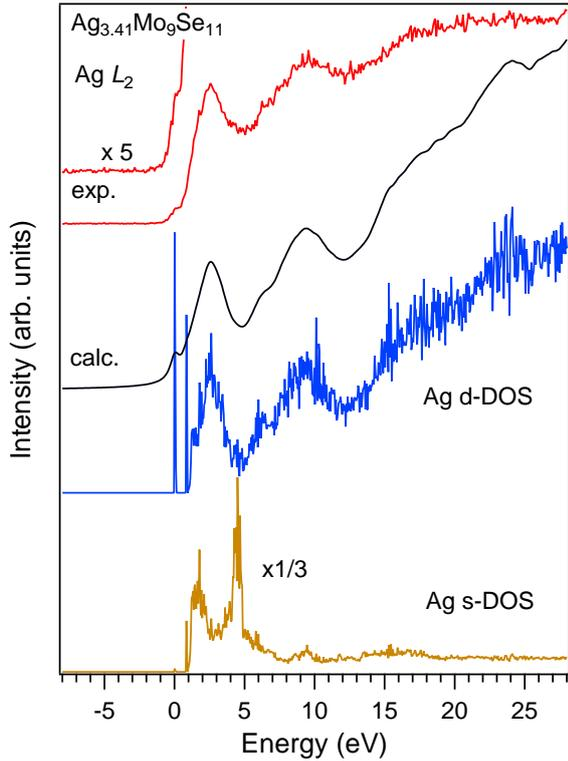
FIG. 8: Experimental Ag  $L_2$  XAS spectrum of  $\text{Ag}_{3.41}\text{Mo}_9\text{Se}_{11}$  compared to the calculated spectrum and unoccupied Ag  $d$ - and  $s$ -DOS of  $\text{Ag}_{3.5}\text{Mo}_9\text{Se}_{11}$ . The calculated spectrum is obtained by broadening the Ag  $d$ -DOS to account for experimental resolution.
