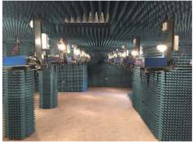
Fig. 2. R2lab Located in an Anechoic Chamber
