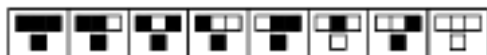
Fig.1. A rule as an application from all possible triplets of cell states to the two possible cell states.
