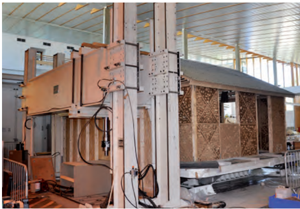
Below: hydraulic jack activating the vibrating table
