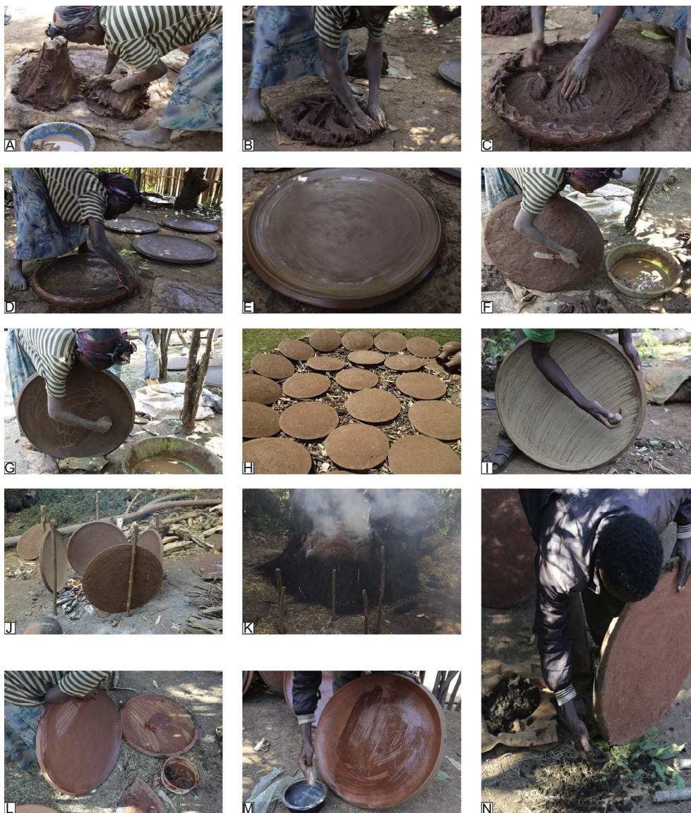
Fig. 4. The Woloyta Chaîne opératoire for making the flatbread dish (called bashe ). (A) Mixing of clay. (B) Modeling from a lump of clay by horizontal drawing. (C) Addition of clay in the centre of the dish. (D) Shaping the rim with continuous pressures. (E) The dish after shaping. (F) Shaving the outer surface with a metal knife. (G) Smoothing the inner face with a piece of cloth soaked in water. (H) Sun drying before pre-firing. (I) Burnishing the inner face with a small pebble for facilitating the adherence of coatings. (J) Pre-firing. (K) Open firing; combustible includes wood and straw. (L) Coating the inner face with a red slip. (M) Coating the inner face with a mixture of water and Abyssinian banana tree roots. (N) Coating the edge of the dish with animal dung.
