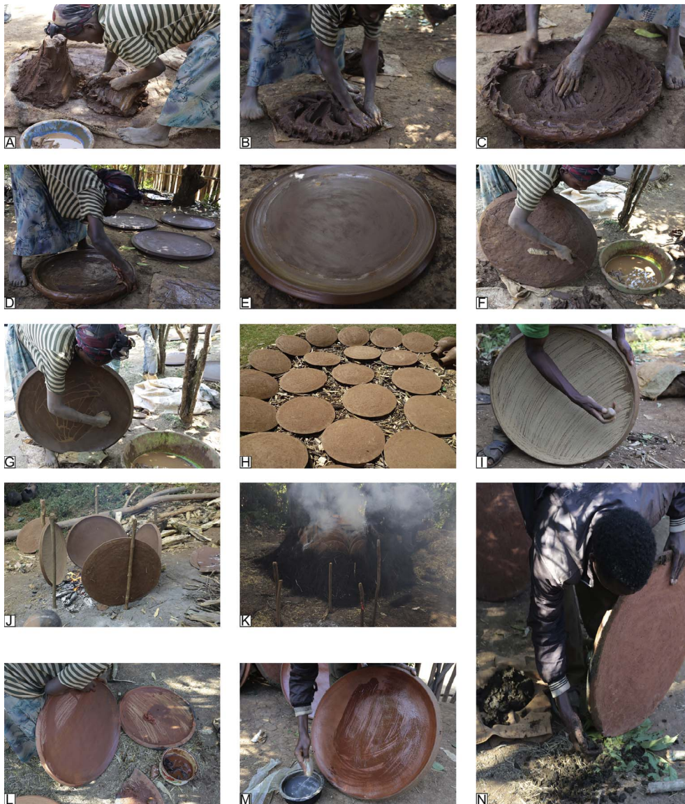
Fig. 4. The Woloyta Chaîne opératoire for making the flatbread dish (called basha ). (A) Mixing of clay. (B) Modeling from a lump of clay by horizontal drawing. (C) Addition of clay in the centre of the dish. (D) Shaping the rim with continuous pressures. (E) The dish after shaping. (F) Shaving the outer surface with a metal knife. (G) Smoothing the inner face with a piece of cloth soaked in water. (H) Sun drying before pre-firing. (I) Burnishing the inner face with a small pebble for facilitating the adherence of coatings. (J) Pre-firing. (K) Open firing; combustible includes wood and straw. (L) Coating the inner face with a red slip. (M) Coating the inner face with a mixture of water and Abyssinian banana tree roots. (N) Coating the edge of the dish with animal dung.
