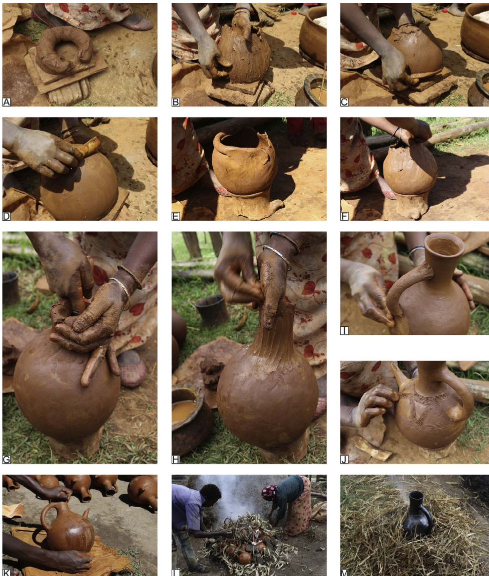
Fig. 3. The Oromo Chaîne opératoire for making the cafetiere (called jabana ). (A) Starting with a thick coil. (B) Drawing the walls with upward discontinuous pressures. (C) Shaping by scraping with a bone spatula. (D) Closing the bottom. (E) Adding a coil for making the shoulder of the cafetiere. (F) Shaping the shoulder. (G) Adding a coil for making the neck. (H) Shaping the neck. (I) After finishing the neck, attaching the handle. (J) Incising decors with a comb on wet surfaces. (K) Coating the Jabana with a polish made out of red clay slip mixed with water and vegetable oil or diesel. (L) Open firing; combustible includes wood, twigs and dried dung. (M) Coating the outer surface with carbon by smoking it out; this is done by plunging the hot cafetiere into straw.
