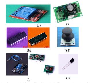
**Figure 3:** Robotic Electrical and Electronic Components. (a) Arduino Module Relay SRD 5 VDC-2 Channels. (b) DC-DC electronic converter. (c) Decoder and Encoder. (d) Joystick Drive. (e) Arduino UNO, Receiver module (Rx) and Transmitter module (Tx), respectively. (f) Photodiode Utilized for the Alarm System.
