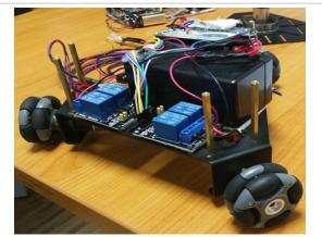
Figure 2: The Robotic Mechanical Base Description, Omni Wheel Chassis Holding DC Motors.
