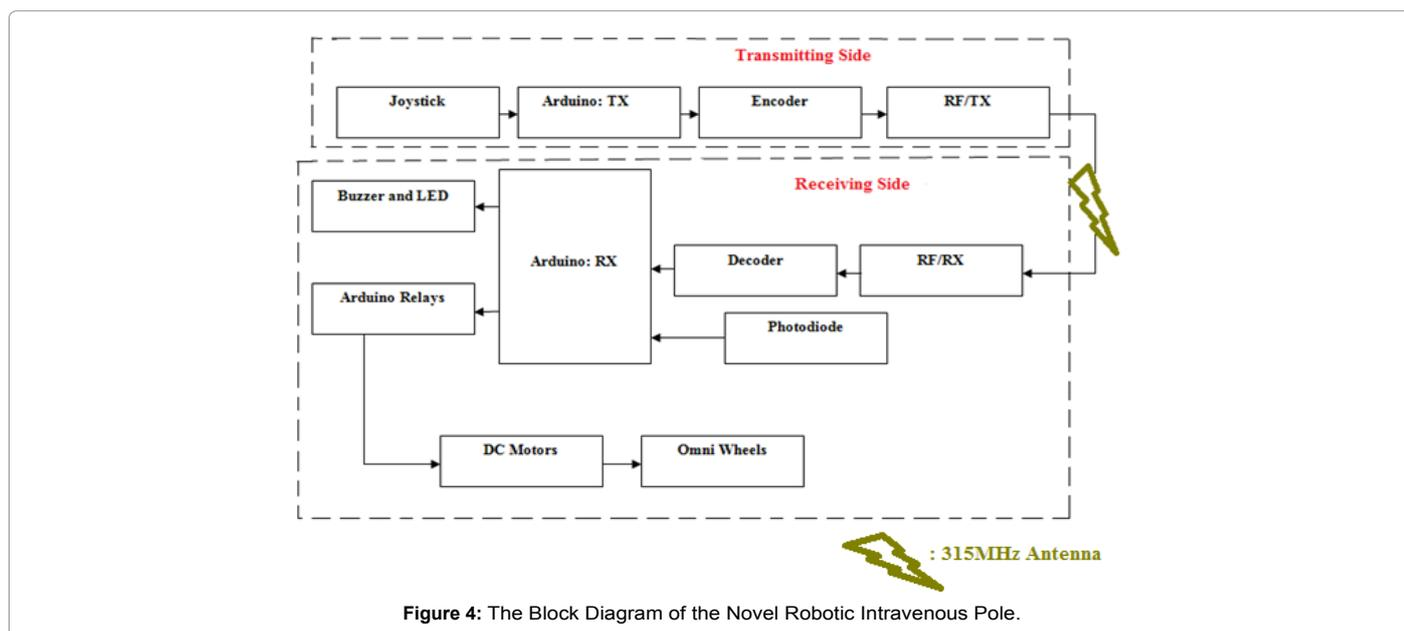
Figure 4: The Block Diagram of the Novel Robotic Intravenous Pole.
