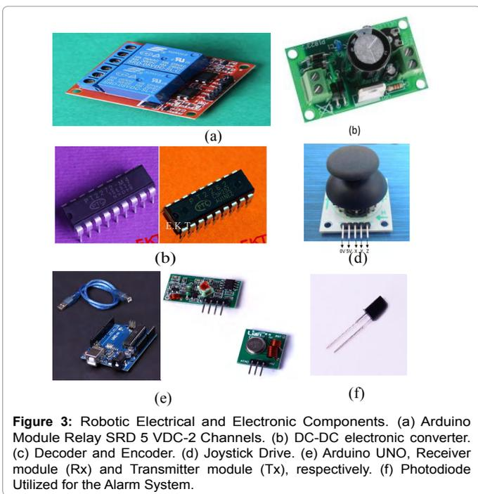
**Figure 3:** Robotic Electrical and Electronic Components. (a) Arduino Module Relay SRD 5 VDC-2 Channels. (b) DC-DC electronic converter. (c) Decoder and Encoder. (d) Joystick Drive. (e) Arduino UNO, Receiver module (Rx) and Transmitter module (Tx), respectively. (f) Photodiode Utilized for the Alarm System.
