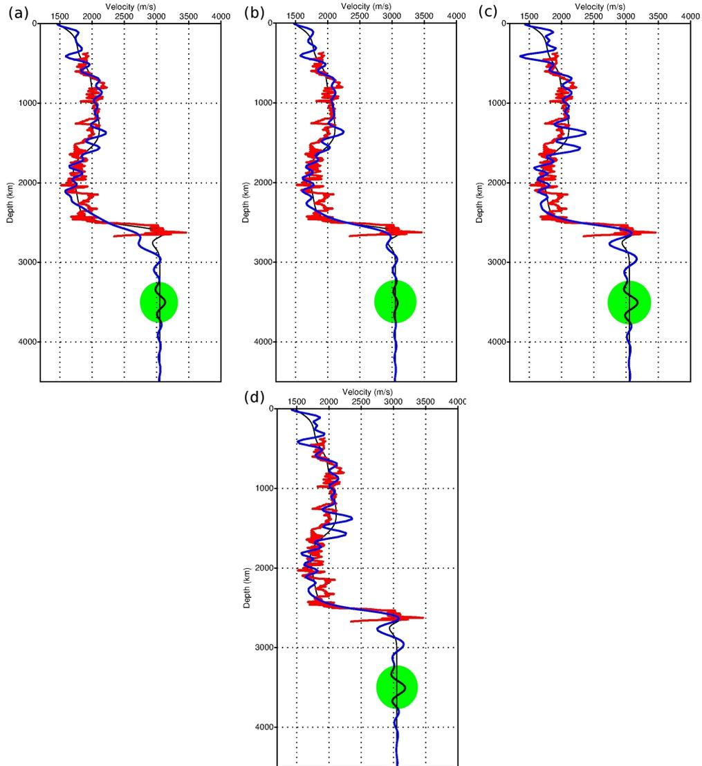
**Figure 8.** P-wave velocity logs compared to a reference well-log at  $x = 9.5$  km, with *strong* regularization. Results obtained using the nonlinear conjugate gradient (a), *l*-BFGS (b), truncated Gauss-Newton (c), truncated Newton (d)
