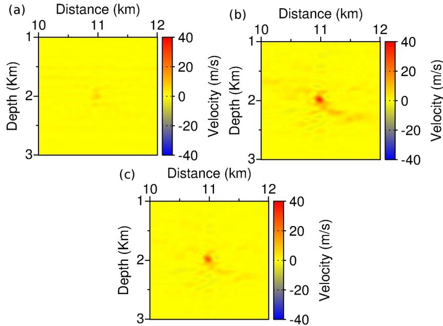
**Figure 10.** Reconstruction of a small amplitude perturbation in the final estimation. Zoom on the perturbation. Nonlinear conjugate gradient (a), truncated Newton method with 3 inner linear iterations (b), 7 inner linear iterations (c)
