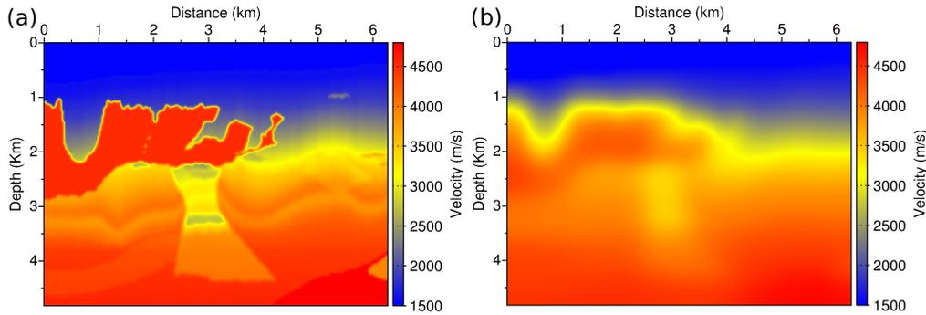
**Figure 1.** BP 2004 synthetic exact model (a), initial model (b).
