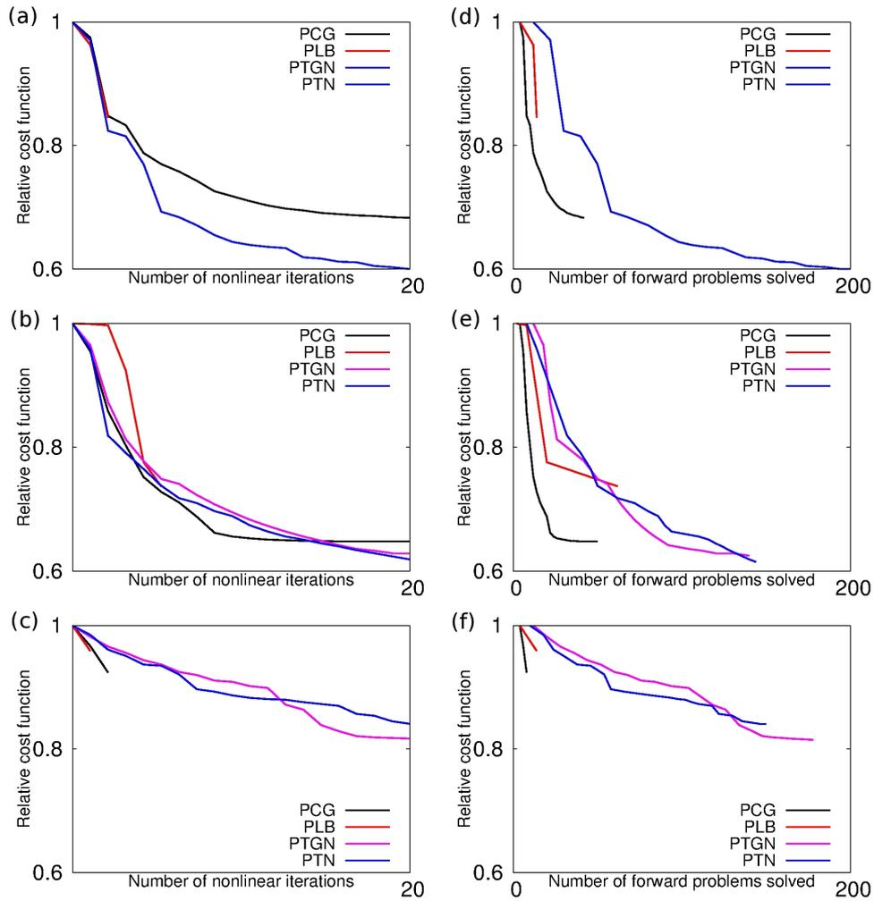
**Figure 11.** Misfit function decrease for the Valhall case study for the *strong* regularization case. Decrease with respect to the number of nonlinear iterations: frequency group 1 (a), frequency group 3 (b), and frequency group 5 (c). Decrease with respect to the number of wave equation problems solved: frequency group 1 (d), frequency group 3 (e), and frequency group 5 (f). PCG: nonlinear conjugate gradient, PLB: *l*-BFGS, PTGN: truncated Gauss-Newton method, PTN: truncated Newton.
