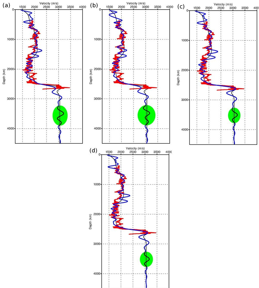
**Figure 7.** P-wave velocity logs compared to a reference well-log at  $x = 9.5$  km, with *weak* regularization. Results obtained using the nonlinear conjugate gradient (a), *l*-BFGS (b), truncated Gauss-Newton (c), truncated Newton (d)
