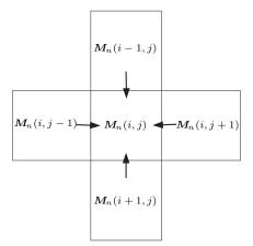
Fig. 4: Schematic illustration of the spatial regularization.  $M_n(i, j)$  represents the abundance of the *n*-th endmember for the (i, j)-th pixel. Each of the four neighbors imposes a spatial regularization effect on the center pixel.
