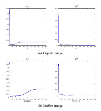
Fig. 6: Influence on the reconstruction errors of the Gaussian bandwidth parameter  $\sigma$  for the unconstrained kernel-NMF with the multiplicative update rules.
