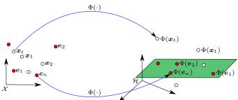
Fig. 3: Illustration of the kernel-NMF proposed in this paper. As opposed to the one shown in Fig. 2, the proposed approach estimates the elements  $e_n$  for n = 1, 2, ..., N directly in the input space  $\mathcal{X}$ , which is the input space of observations. This strategy allows us to overcome the curse of the pre-image problem, by estimating directly the spectra.
