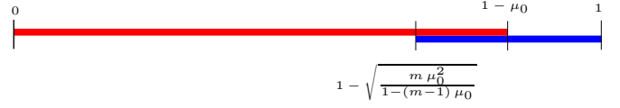
Fig. 2. Squared error bounds of approximating a kernel function from a \mu_0 -coherent dictionary of size m . The blue region corresponds to the kernel functions verifying (6), while the red one to its violation.
