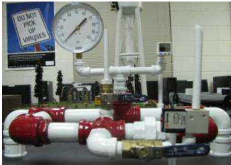
Fig. 1. Gas pipeline testbed
