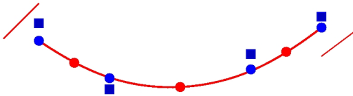
Figure 3: Step 2: computation of the flux from the solution at flux points. Without treatment, two different fluxes are found at segment end points.
