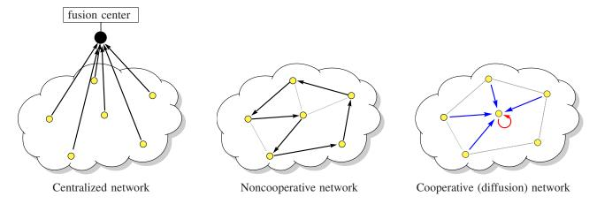
Fig. 1. Illustration of information processing in a network: While the centralized network requires a fusion center, the noncooperative and cooperative networks provide in-network processing. The noncooperative network process the information by using a given routing path. The cooperation network operates information diffusion, using either a combine-then-adapt or an adapt-then-combine strategy.
