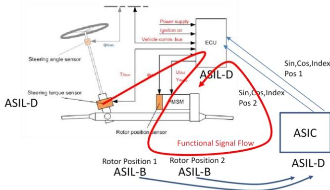
Figure 1. Signal flow analysis of the EPS system.
