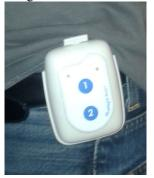
Figure 1. The ACOR+ is an IMU with reduced dimensions (77x57x25 mm) and light weight (70 g) to be clipped on the belt.
