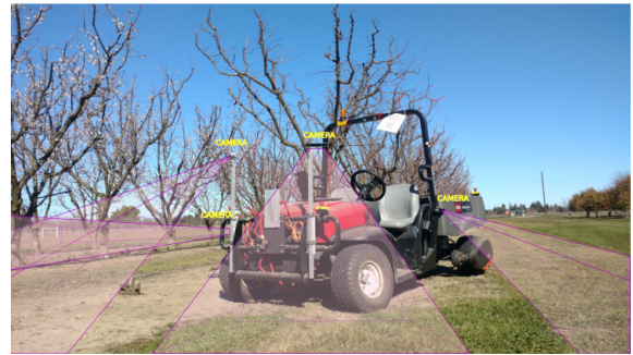
Fig. 2. Toro workman MDE vehicle equipped with 4 stereo cameras
