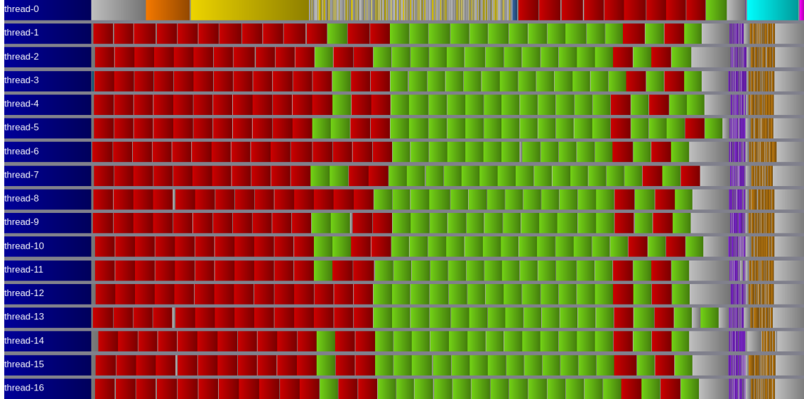
Figure 4: Task scheduling of one iteration of the task variant within only one MPI process using on 16 nodes. The legend is same than Figure ??.
