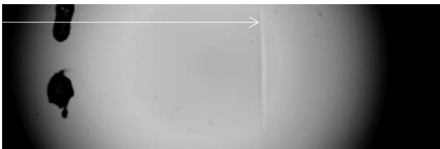
Fig. 8 Shockwave detected by direct shadowgraphy in zoomed view.
