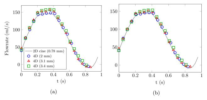
**FIGURE 2** Inlet flow waveforms over one cycle measured at different isotropic voxel sizes (a) without and (b) with near-wall velocity masking.
