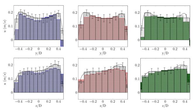
**FIGURE 7** Axial velocity profiles in the middle of the bend (see Figure 1 a) along y (right-left) and z (foot-head) axis; (— ) HR-CFD. Grey filled bar chart LR-CFD; 1st/2nd/3rd columns: 2 mm/3.1 mm/3.4 mm voxel size 4D Flow MRI acquisitions respectively. Error bars correspond to  $u \pm u_{rms}$
