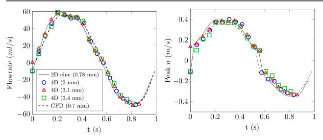
FIGURE 6 left Flowrate and right peak axial velocity evolution over one cycle in the collateral branch (see Figure 1 a).
