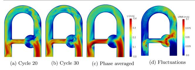
**FIGURE 4** Magnitude velocity fields in the flow phantom at peak systole for cycle 20 (a), cycle 30 (b), phase-averaged (c). The velocity fluctuations (d) are expressed through  $\mathbf{u}_{rms}$ . Important cycle-to-cycle fluctuations between the instantaneous fields indicate non reproducible disturbed zones, where turbulence is more likely to appear, while the phase averaged field encompasses dominant flow patterns.
