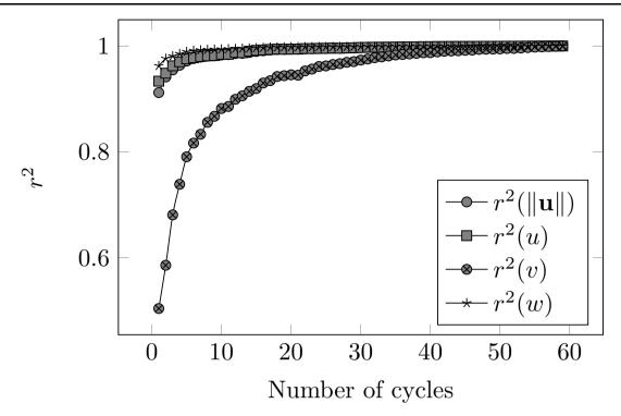
**FIGURE 3** Evolution of the Pearson's correlations ( $r^2$ ) between phase-averaged CFD velocity computed over different numbers of cycles the and 60-cycle phase-averaged CFD velocity. The correlations are performed on each node of the domain.
