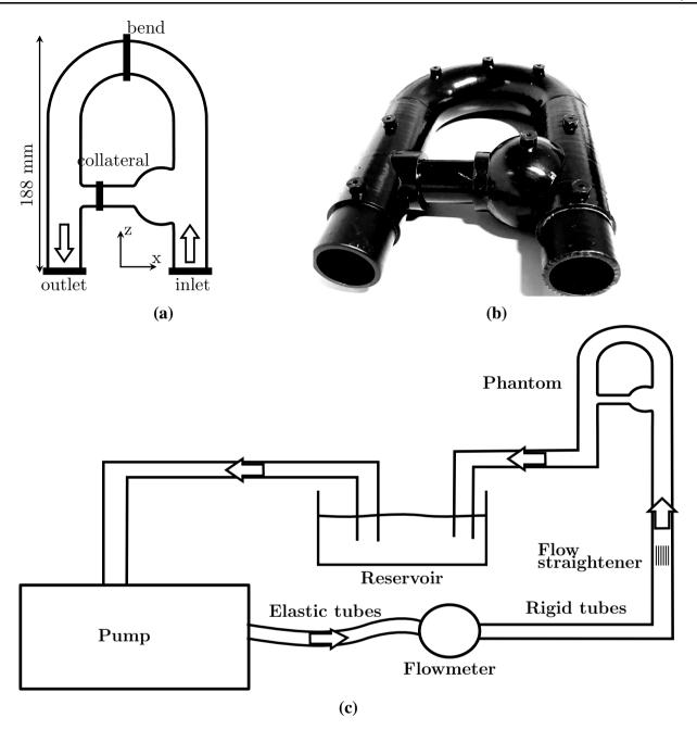
**FIGURE 1** (a) Flow phantom schematic representation in the coronal plane annotated with locations of surfaces of interest. (b) 3D printed flow phantom. (c) Schematic diagram of the experimental setup.
