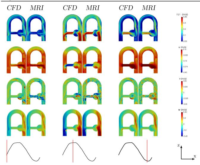
**FIGURE 5** Comparison in the coronal plane of CFD velocity fields with MRI measurements at 2 mm resolution at different instants of the cycle. First row represents the velocity magnitude, while second, third and last rows depict right-left (*u*), up-down (*v*) and foot-head (*w*) velocity components respectively.
