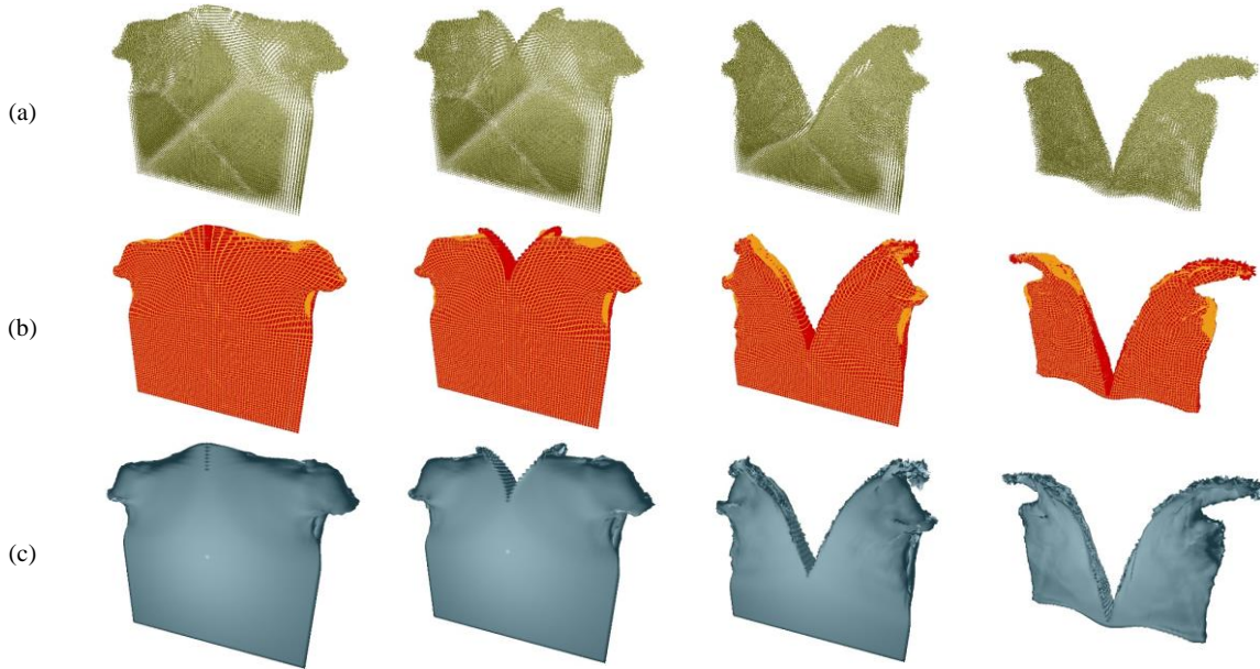
Figure 7: Tearing of a very deformable thin matter bloc. A tearing line is favoured by employing lower Sensor threshold in the centre of the physical model. (a) Direct representation of the physical model, by using a sphere on each mass. (b) Representation of the topological model, in which sewed and unsewed faces are rendered with distinct colours, allowing to pursue the evolving topological modifications. (c) Rendering of the finally obtained geometrical model.
