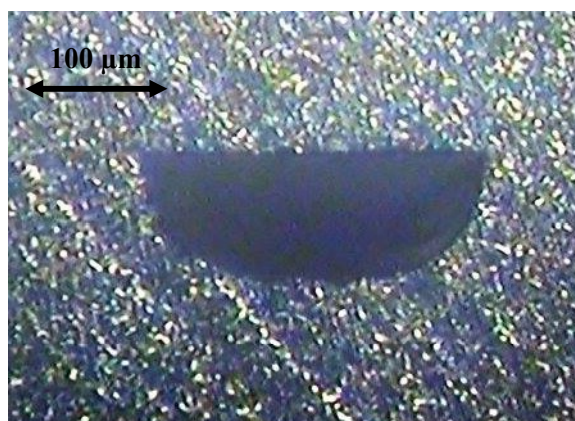
Figure 10. Cross-sectional photograph of a fluidic access channel fabricated with glass etching and bonding procedures.
