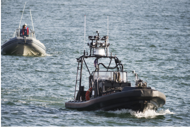
Fig. 5: An Autonomous Surface Vehicle controlled by ASPiC
