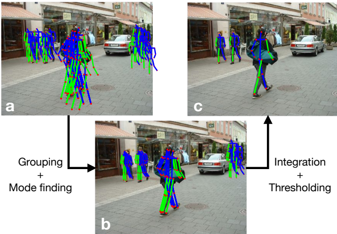
Fig. 5. Illustration of the pose proposal integration (PPI). The pose proposals (a) are grouped based on 2D overlap and 3D pose to identify the persons and the modes (b). Final pose estimates (c) are obtained by averaging the 2D poses in the selected modes and thresholding.
