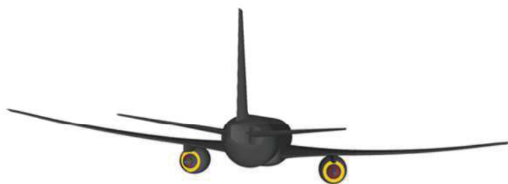
Fig. 4 CRM wing/body/engine geometry used in the simulations, highlighting engine primary core (red) and bypass flow (orange)
