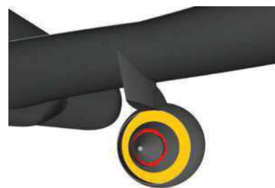
Fig. 5 Close-up of the engine primary core (red) and bypass flow (orange)
