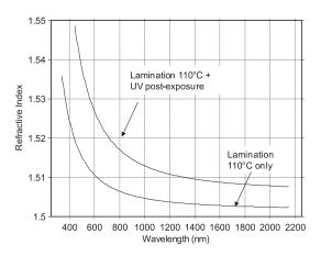
Fig. 4. Refractive index of Ordyl SY317 after 5 passes ot hot roll lamination perfomed at 110 °C. The refractive index can be modulated by post-lamination UV exposure that enhances the cross-linking degree of the polymer typically from 1.503 to 1.510 at a wavelength of 1310 nm.
