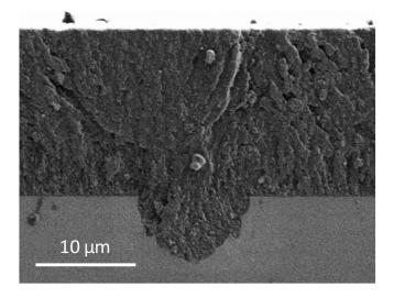
Fig. 3. SEM cross-section of a micro-groove after lamination of an ORDYL SY317 dry film with a roll temperature of 110 °C. Five passes of lamination were applied at a pressure corresponding to a static load of 12 kg. A HMDS adhesion promoter was vapor-stream-deposited prior to the dry film application.
