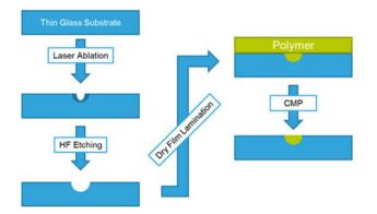
Fig. 1. Fabrication sequence of surface U-shaped optical guide in a thin glass substrate: i) localized laser-induced modification of glass microstructure, ii) U-groove etching based on locally enhanced HF etching rate, iii) dry film polymer lamination to fill the groove and iv) planarization of the core material using CMP.
