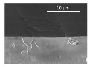
Fig. 6. SEM picture showing a cross-section of a surface waveguide after the CMP step. The core hemicylinder is composed of ORDYL SY317, the bottom cladding is a glass substrate AF32 Eco.
