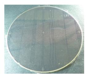
Fig. 5. Picture showing a 3 inches 500  $\mu$ m thick AF32 Eco glass substrate after laser inscription, HF etching and lamination of a ORDYL SY317 dry film. The layout contains straight and bent waveguides as well as Y junctions.
