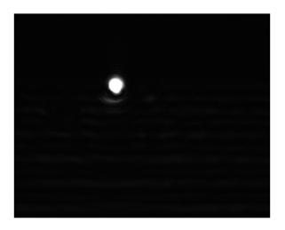
Fig. 8. Mode profile of a waveguide at 1550 nm.
