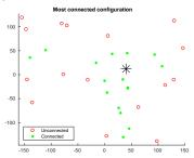
Fig. 9. The most connected configuration (50.00% connected) of a Poisson point process with density  $\lambda=0.001$  and  $\tau=-60$  (or  $\tau_{\lambda}=-30$ ) dB.
