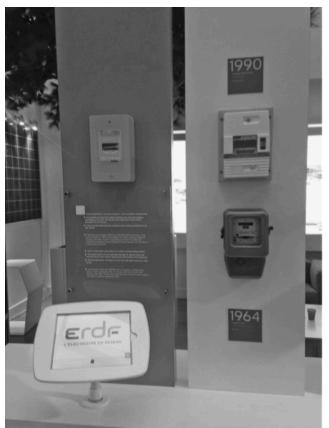
FIGURE 13.3 Electronic meters, introduced into homes in 1990 (right, at the top). We can also see one smart meter Linky (left). From 'The saga of the meter', electric meters in the exhibition showroom of the French electric distributor Enedis in Paris. Personal photograph.
