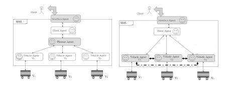
Fig. 1. Centralized architecture (left) and decentralized architecture (right)
