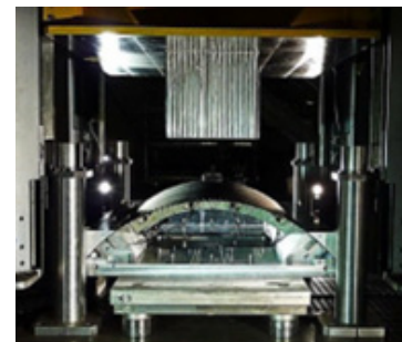
Figure 9 – Pictures of the ONERA test protocols used during the EU SMAES project for static buckling (left) and to mimic crash tests on water (ditching) using equivalent dynamic tests with calibrated honeycombs (right)
