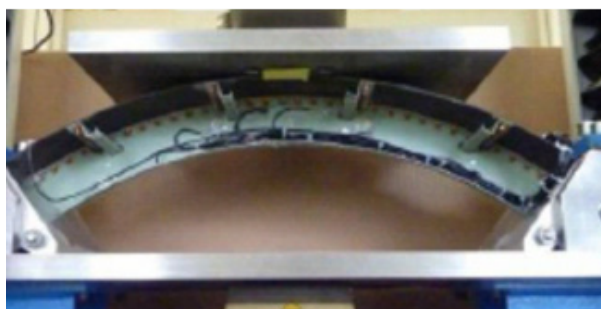
Figure 9 – Pictures of the ONERA test protocols used during the EU SMAES project for static buckling (left) and to mimic crash tests on water (ditching) using equivalent dynamic tests with calibrated honeycombs (right)
