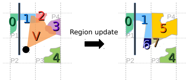
Fig. 8. Update procedure. the robot is in proto-region P_2 but the field of view V covers proto-regions P_1 to P_4 . In P_2 , no regions were previously defined, so a new region is created (region 6). In P_3 , region 4 already existed but has no overlap with V : a new region is created (region 7). Region 1 in P_1 overlaps V , so the region is extended. Lastly, V overlaps two regions in P_4 , so that regions 2 and 3 are merged to create region 5. Last configuration, when a wall is splitting a proto-region, two separate regions are naturally created on each side (as they are not connected components). Thus, region 0 and 1 of P_1 are separated by a wall and cannot be merged together.
