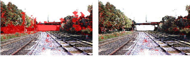
Figure 4: Closeup on HPR results. In red points removed by the HPR: (left) fixed neighborhood, using [PGA11] (right) adaptive neighborhood, using our method.
