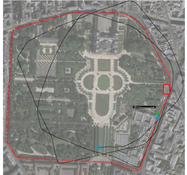
Fig. 1: Trajectory in red of our IMLS SLAM with a vertical Velodyne HDL32 on top of a car (two loops of 2 km length) in the city of Paris. We can see the good superposition of the two loops. In black is the trajectory of the classical scan-to-scan matching. The starting point of both methods is the same green circle. The end point of the IMLS SLAM and the end point of the scan-to-scan matching are inside the blue circles.
