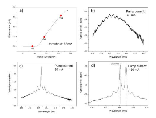
Figure 1 a) L-I curve of the laser. Optical spectra of the diode below (I=40 mA) b), above \$I=90 mA) c) and far above (I=160 mA) d) the laser threshold (I=65 mA).
