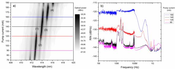
Figure 2 a) Optical spectrum evolution in function of the pump current above the laser threshold. b) RIN measurement for specific current values revealing the impact of mode hopping competition in InGaN laser. Strong peaks between 10 and 30 MHz are contributions from electromagnetic perturbations of the setup
